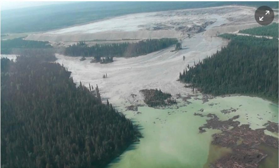
The results of a tailing pond breach at Imperial Metals Corp's gold and copper mine, which released millions of cubic meters of water and waste. Photograph: Reuters
