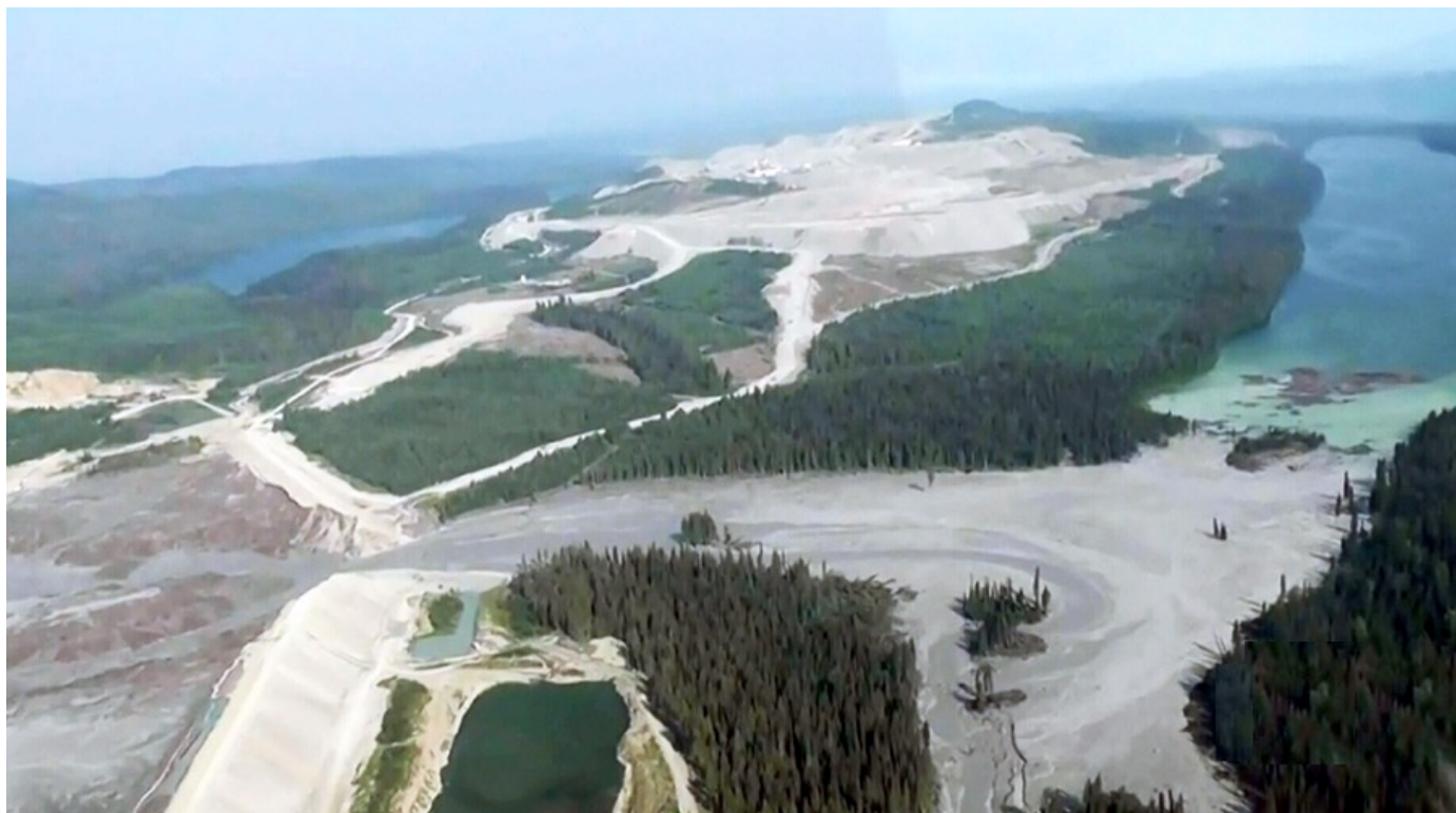
Aerial view of the Mount Polley mine tailings pond shows the area where the dam wall gave way early on the morning of August 4, 2014. Image from archives
